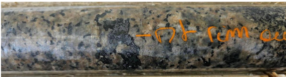
Figure 9: Beige, grey syenite with magnetite crystals at the core or rim around amphibole
