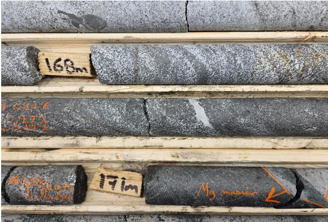
Figure 13: Magnetite layered carbonatite in hole CH-25-04 (168 m)
