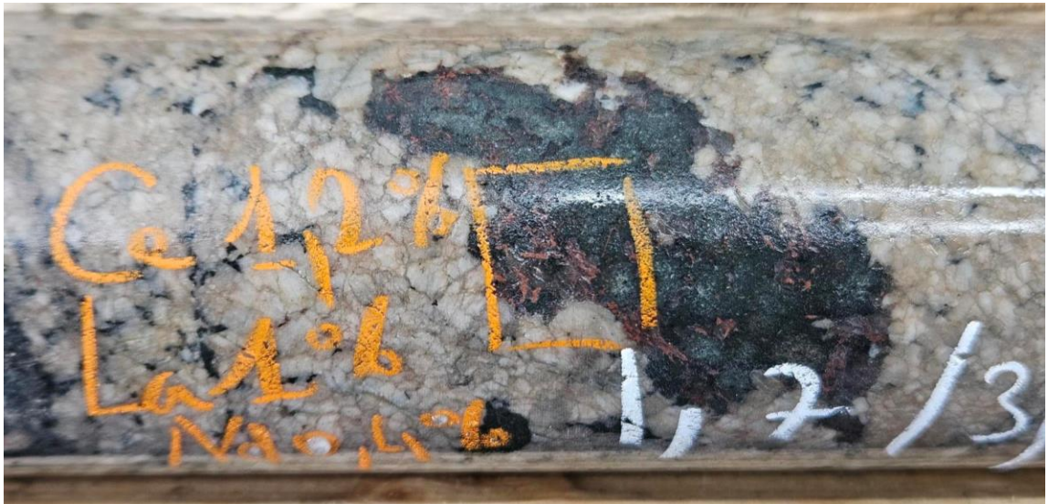
Figure 17: Mafic (amphibole-magnetite) aggregate with dark reddish minerals REE-rich at 32.90 m
