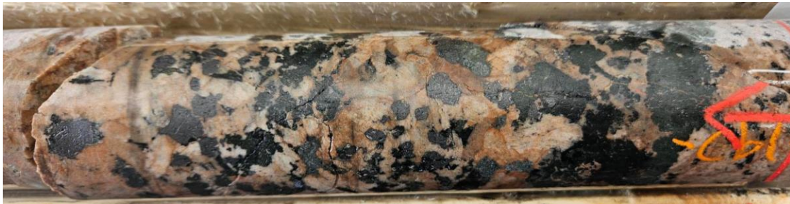
Figure 8: Pinkish to orangish syenite with magnetite and amphibole crystals. That type of interval gives a higher scintillometer response.
